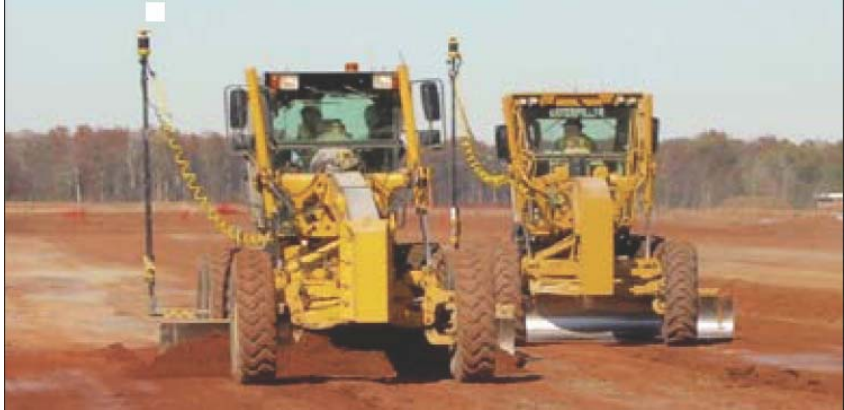
Figure 2.2 – Motor Graders outfitted with 3D Machine Control System from TopCon
