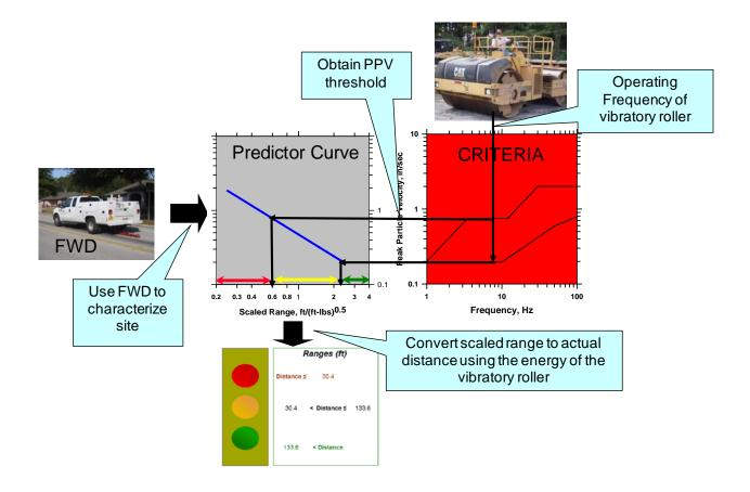
Figure 2 Overall Vibration Analysis Procedure
