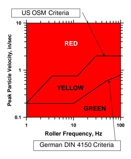
Figure 1 FDOT Adopted Vibration Threshold Criteria
