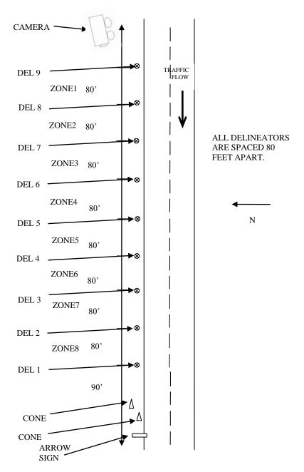
FIGURE 6 Layout of delineator setting in the field.
